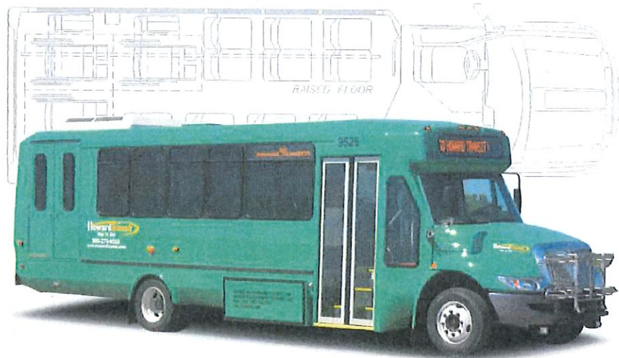
14 Passengers, Perimeter Seating, 72" Luggage Rack, 2 Wheelchair Positions, Rear Lift
