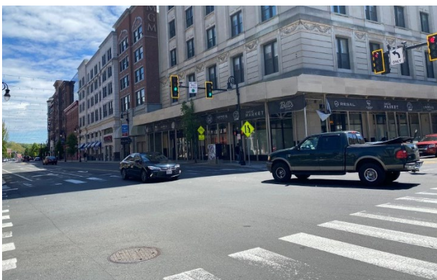
Figure 11. Example of retroreflective backplates installed at State/Main
